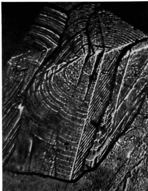
Fig. 4. Sucrose crystal isolated from solution containing dextrose by method 1. (100) face. \times 60 . Step height 4000 Å.
