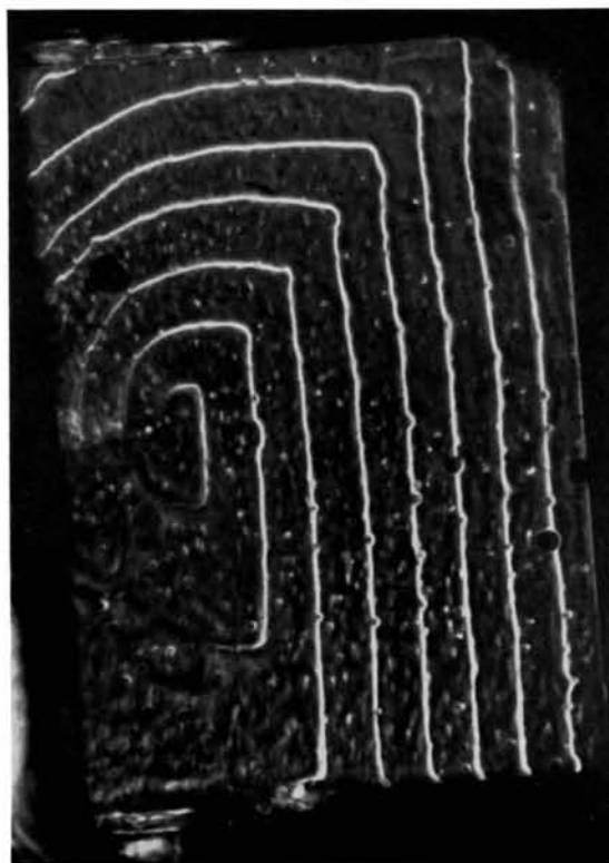
Fig. 5. Sucrose crystal isolated by method 2. (100) face. \times 430 . Step height 1700 Å. Phase contrast.
